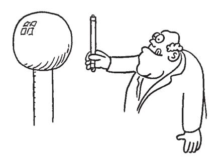
THE LAMP WILL NOT GLOW WHEN IT IS HELD WITH BOTH ENDS EQUIDISTANT FROM THE CHARGED VAN DE GRAAFF GENERATOR. BUT WHEN ONE END IS CLOSER TO THE DOME THAN THE OTHER END, A CURRENT IS ESTABLISHED AND IT GLOWS. WHY?
