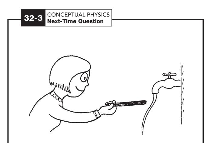
A thin stream of water bends toward a negatively charged rod. When a positively charged rod is placed near the stream, it will bend in the
