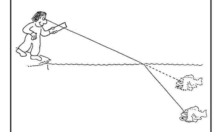
BRUNO WISHES TO "SPEAR" A FISH WITH A LASER. SHOULD HE AIM THE LASER BEAM ABOVE, BELOW, OR DIRECTLY AT THE OBSERVED FISH TO MAKE A DIRECT HIT?
